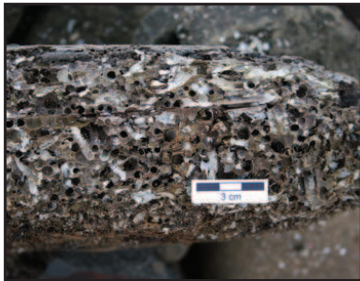
An example of damage from shipworms.
